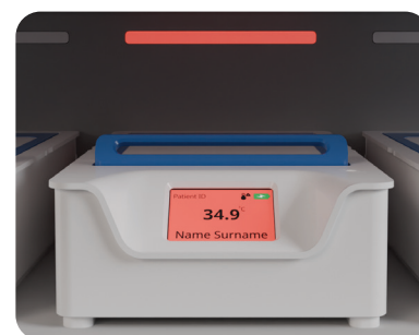
Red LED light indicating an anomaly inside the chamber
